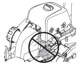
Clean the cooling system with a brush once a week, more often in demanding conditions. A dirty or blocked cooling system results in the machine overheating which causes damage to the piston and cylinder.
